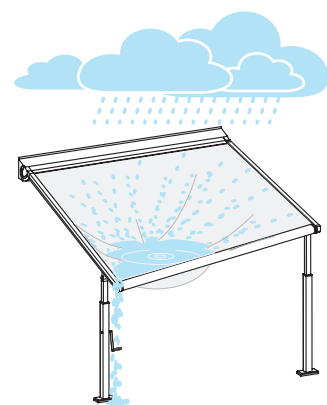
When exceeding rain class 2 (56 l/h/m 2 ), the Plaza Viva must be retracted. Risk of damage!
