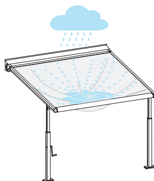
If the post is not lowered, the water may collect on the Plaza Viva leading to pooling.
