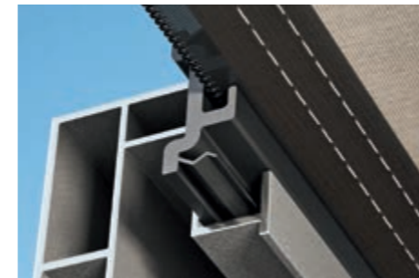
Functioning principle of OptiStretch
